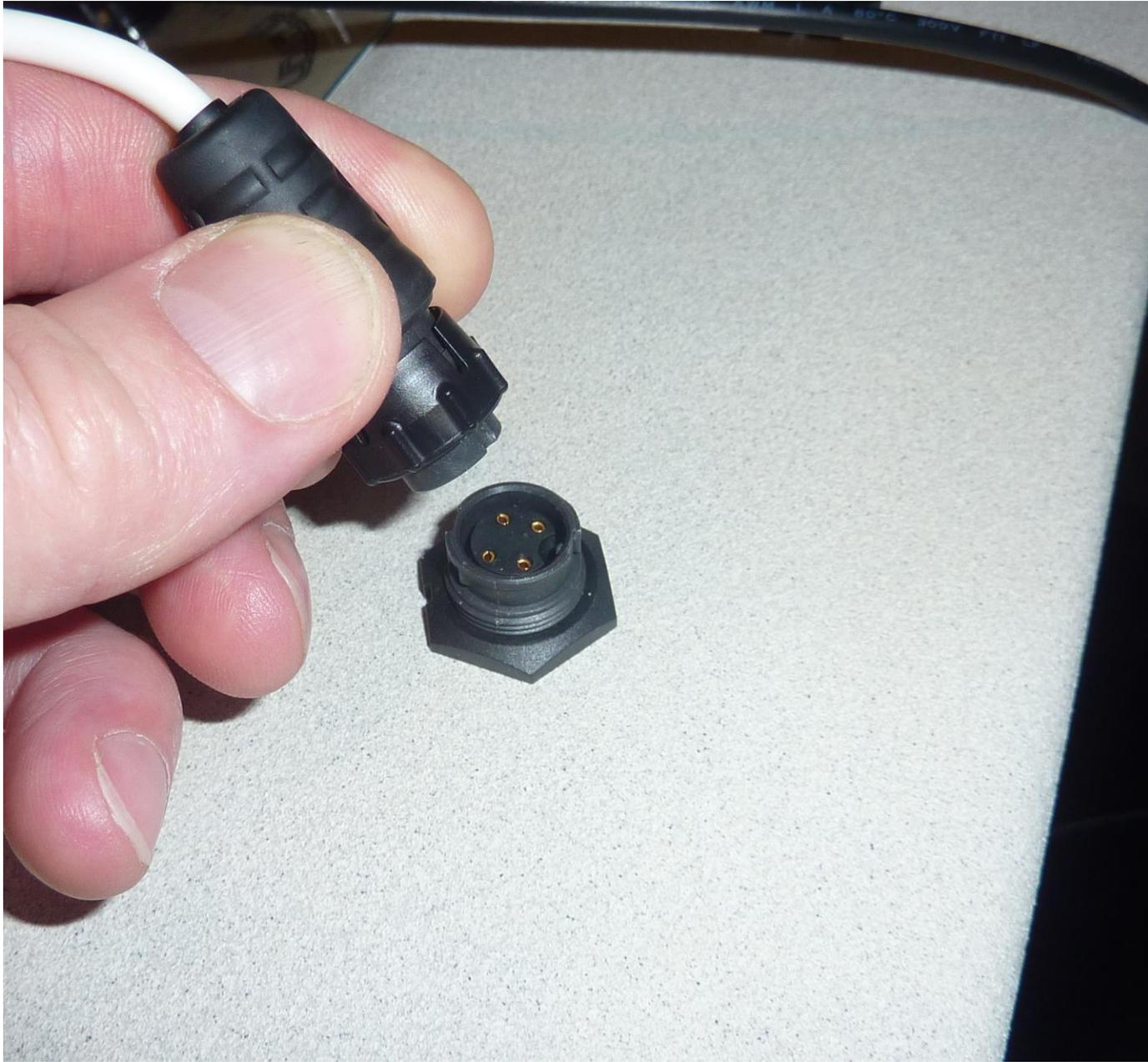
After inserting the plug, turn the collar on the plug clockwise to lock the plug into position.
