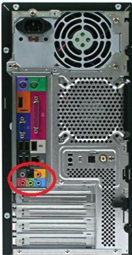
The sound outputs are shown. On this set up, you would typically plug the lead into the green port which is usually the audio "line-out" port. The green port is usually the output on sound cards as well.
